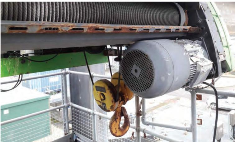
Further corrosion to original hoist steelwork and bottom block assembly
