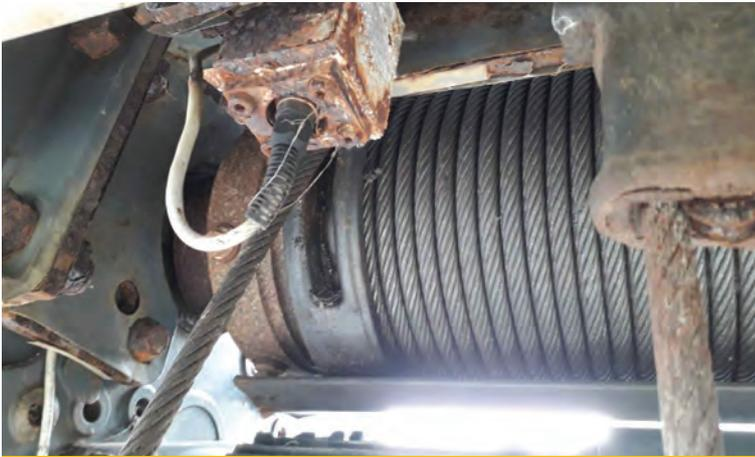
Corroded rope and dead-end assembly on original hoist
